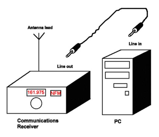
The sound mixer utility software, provided with the soundcard, should be used to select the line input (sometime called aux input) for recording. The volume control (audio level) in the utility should be set at such a level that it avoids saturation of the audio circuitry (often indicated by a green/yellow/red bargraph in the utility).
